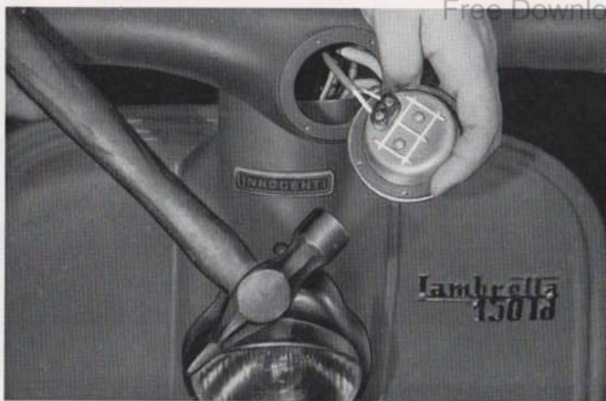
Varying the note of the A.C. horn which has no adjuster
