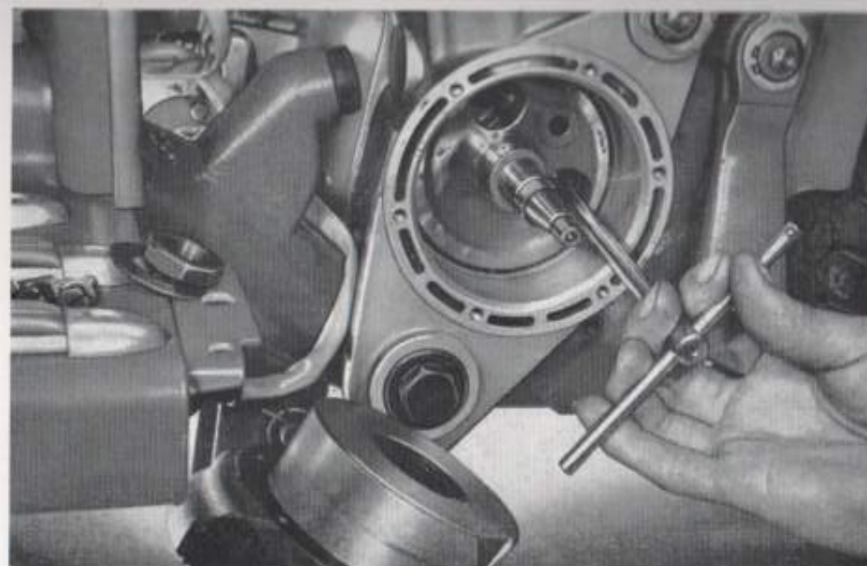
After engine 167530 remove the crankshaft without dismantling the gearbox
