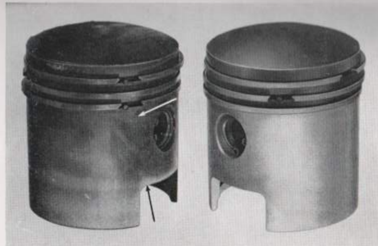
Right piston normal, side of other shows blackening at top and rubbing at bottom indicating a bent connecting rod
