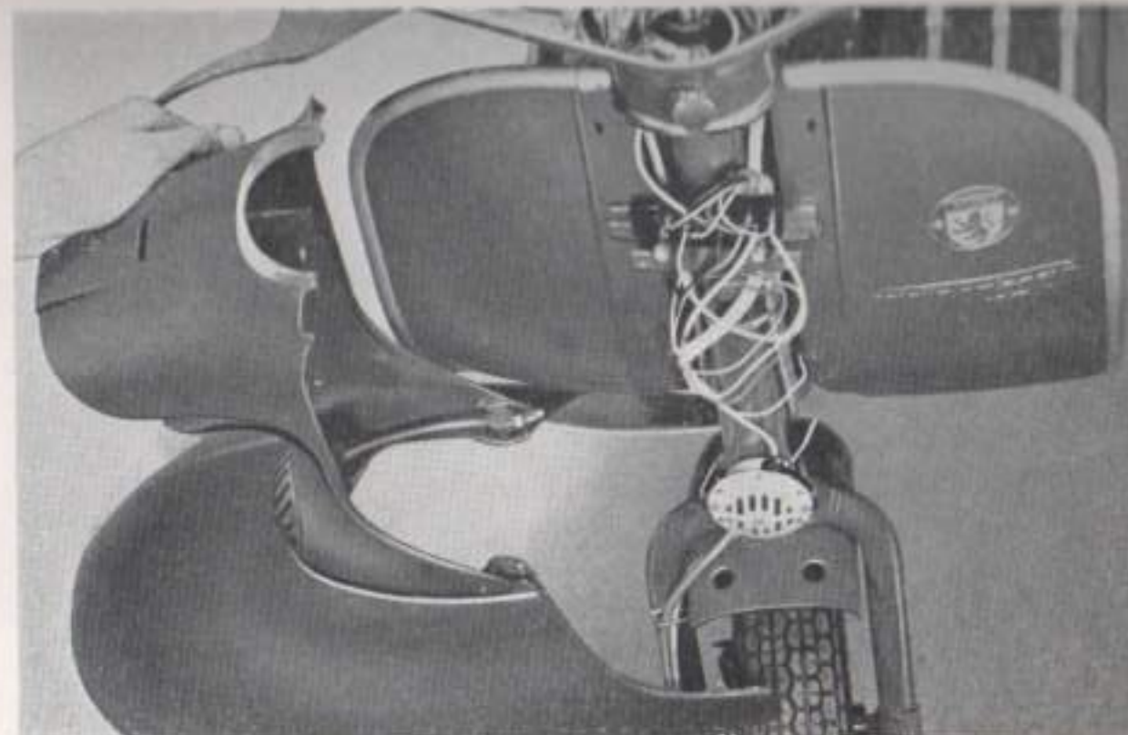
Mudguard and headlamp casting removed to show cables
