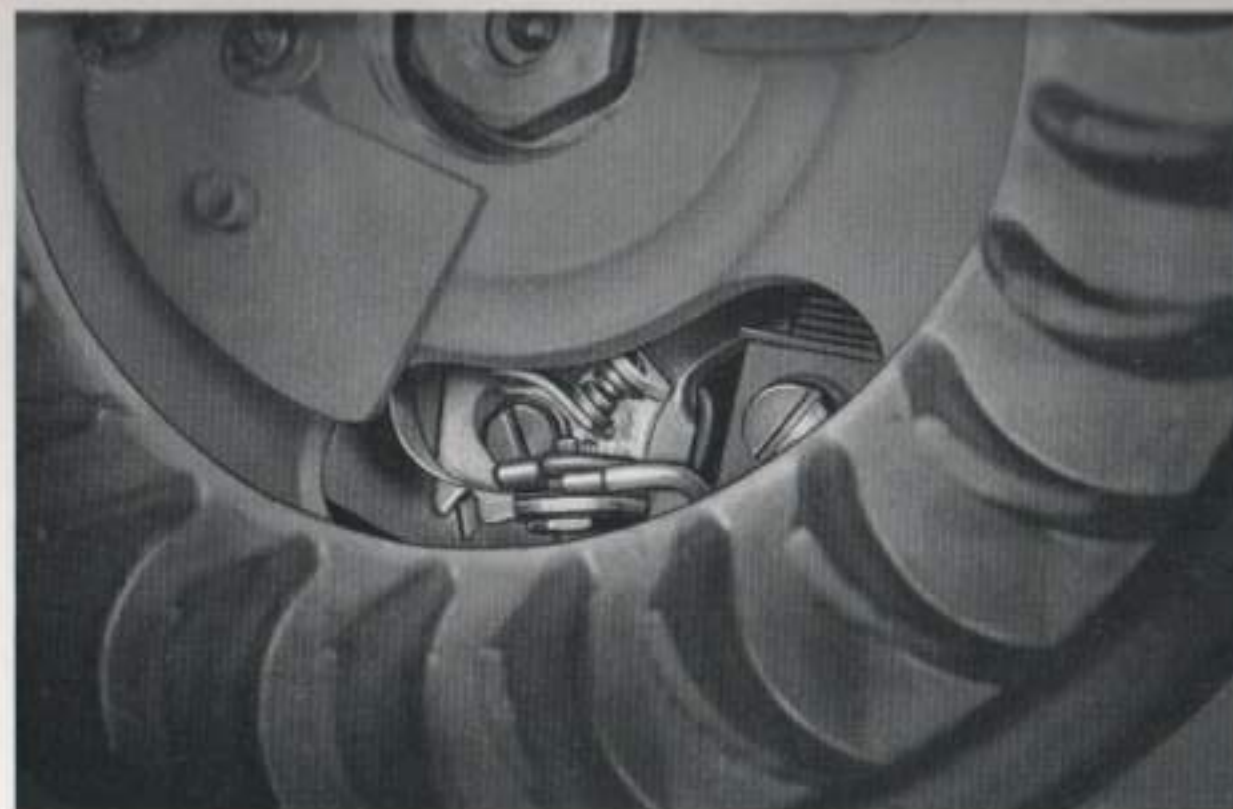
Filso contact points. Note locking screw and V-notch adjustment
