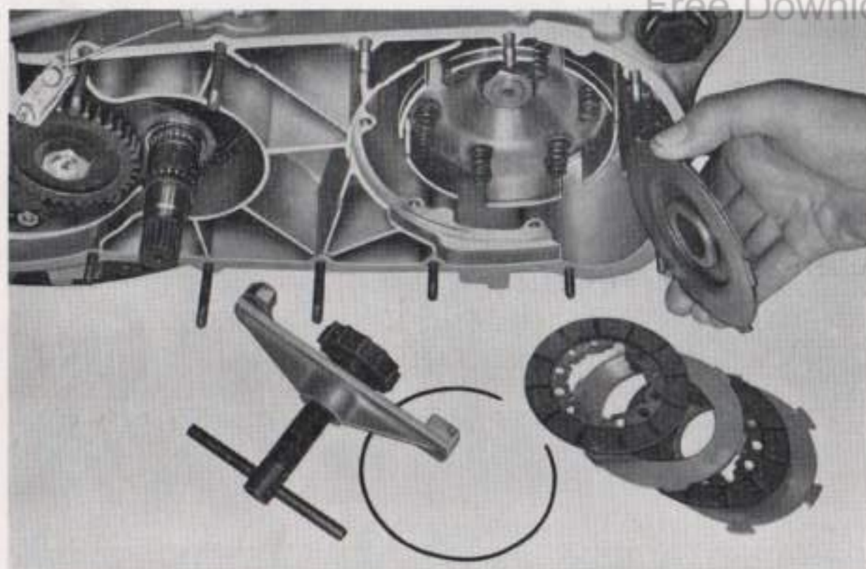
Clutch on crankshaft, compressor and plate aligning tool 56686 in foreground
