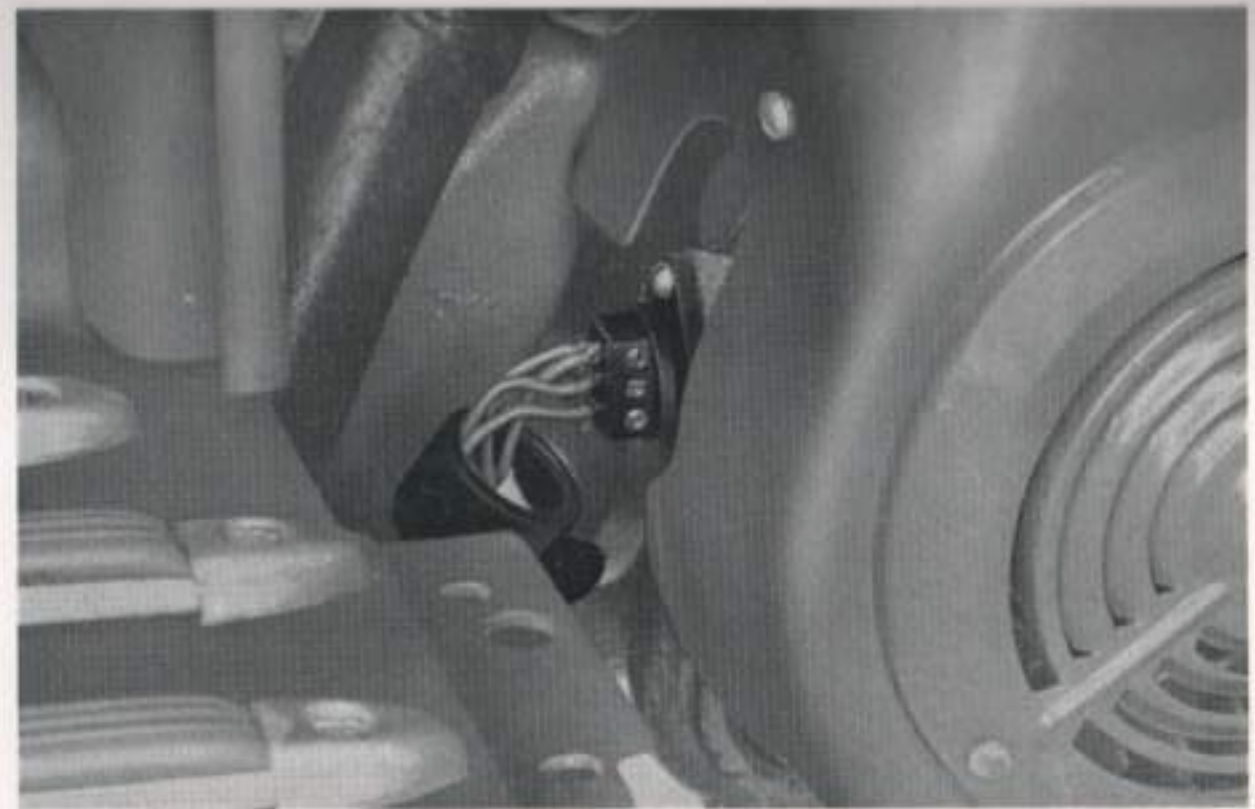
Terminal block on the side of the magneto flange
