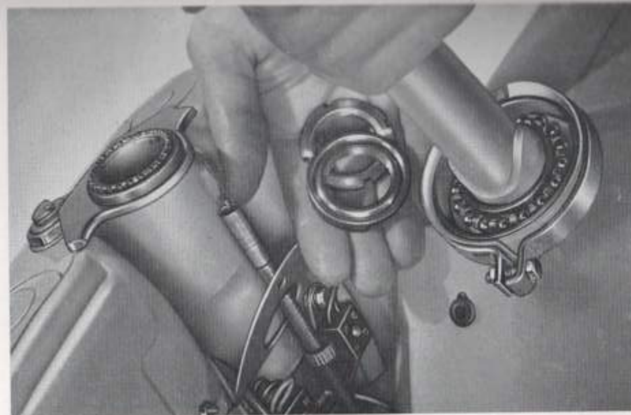
The cup and cone bearings of the steering with caged ball races
