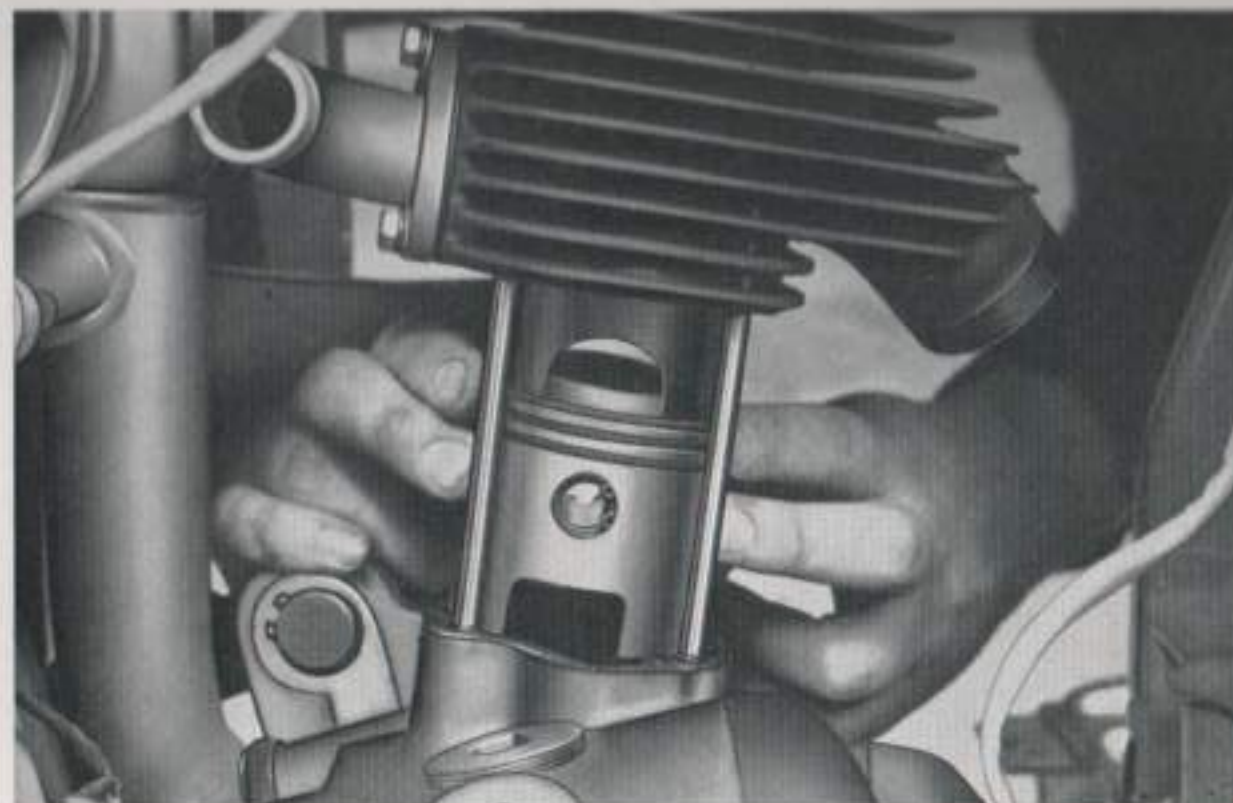
Allow the cylinder to slide on by its own weight while positioning the rings
