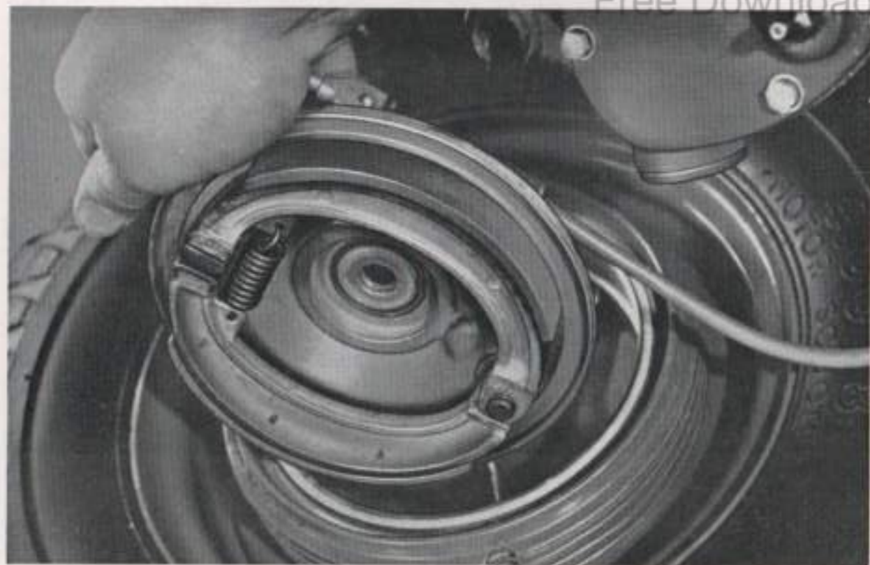
Examining the brake shoes from the front wheel
