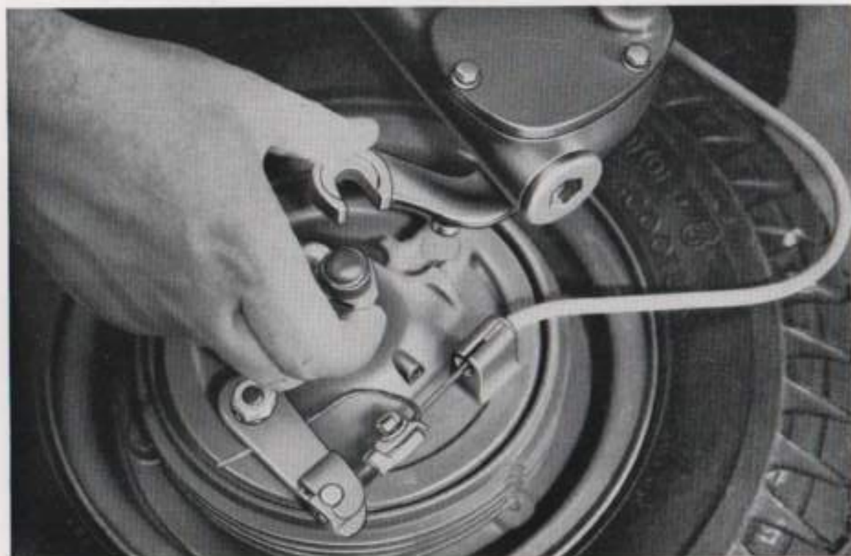
Ensure that the anchor peg engages the slot in the backplate on re-assembly
