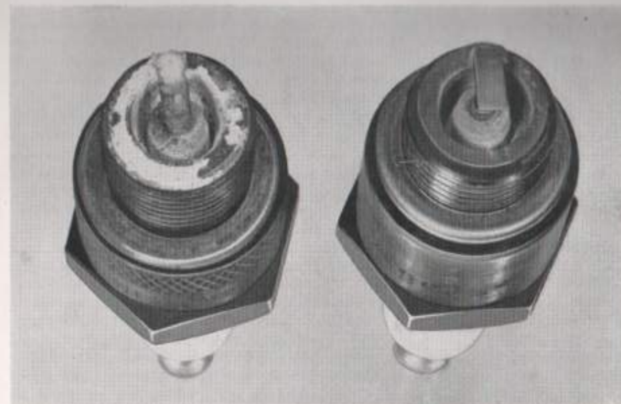
Spark plug on right shows normal condition, that on left is overheating
