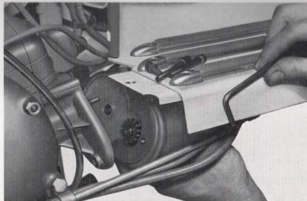
Removing the motor unit using a 5 mm allen key
