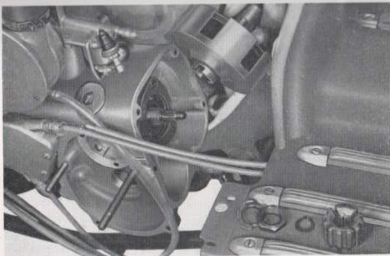
Removing the clutch bell with extractor 39146
