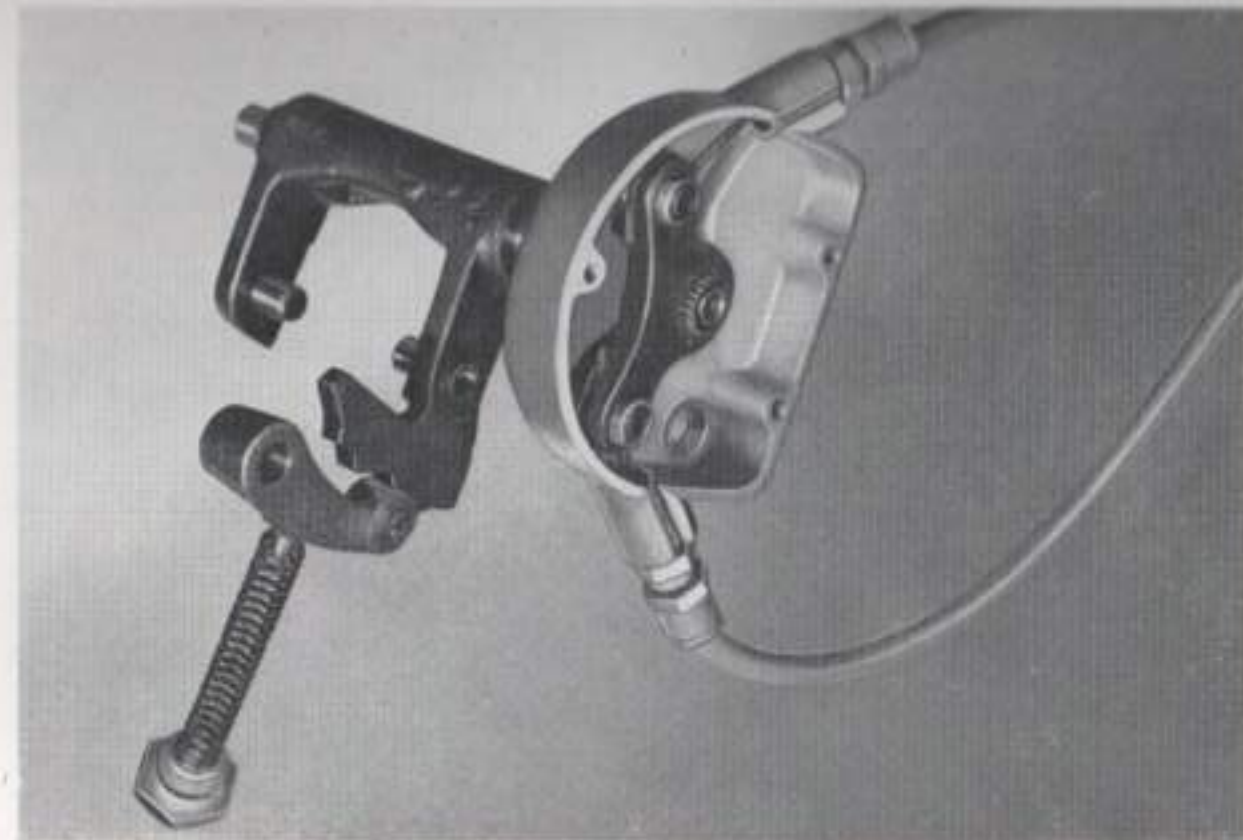
The selector arm and gate operated by the gear change cables
