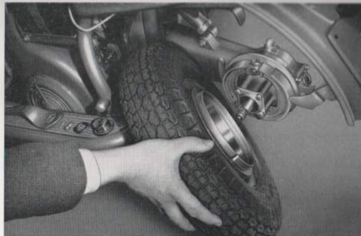
Rear wheel and hub removed for attention to brake shoes
