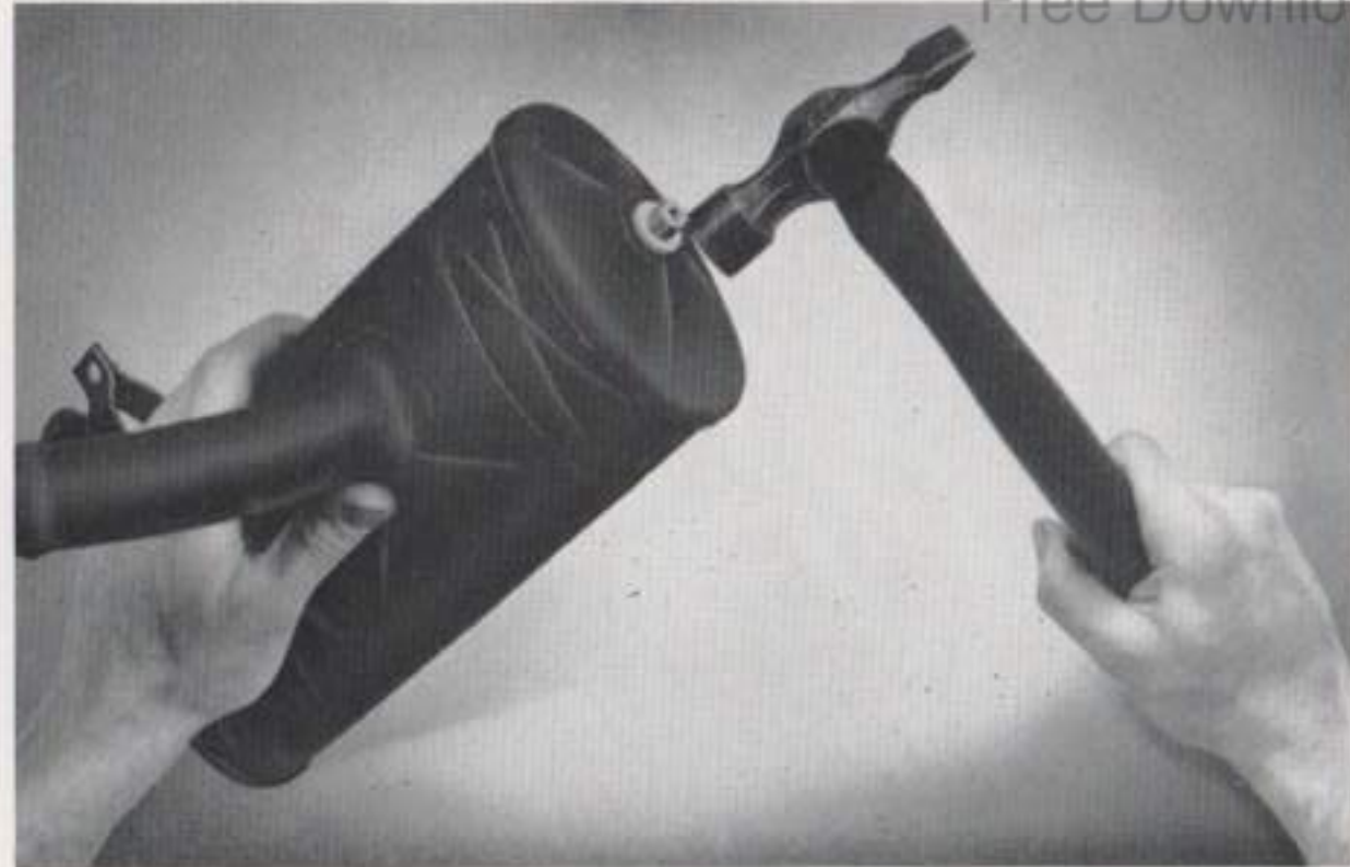
Tapping the silencer end-caps into position to obtain a gas-tight seal
