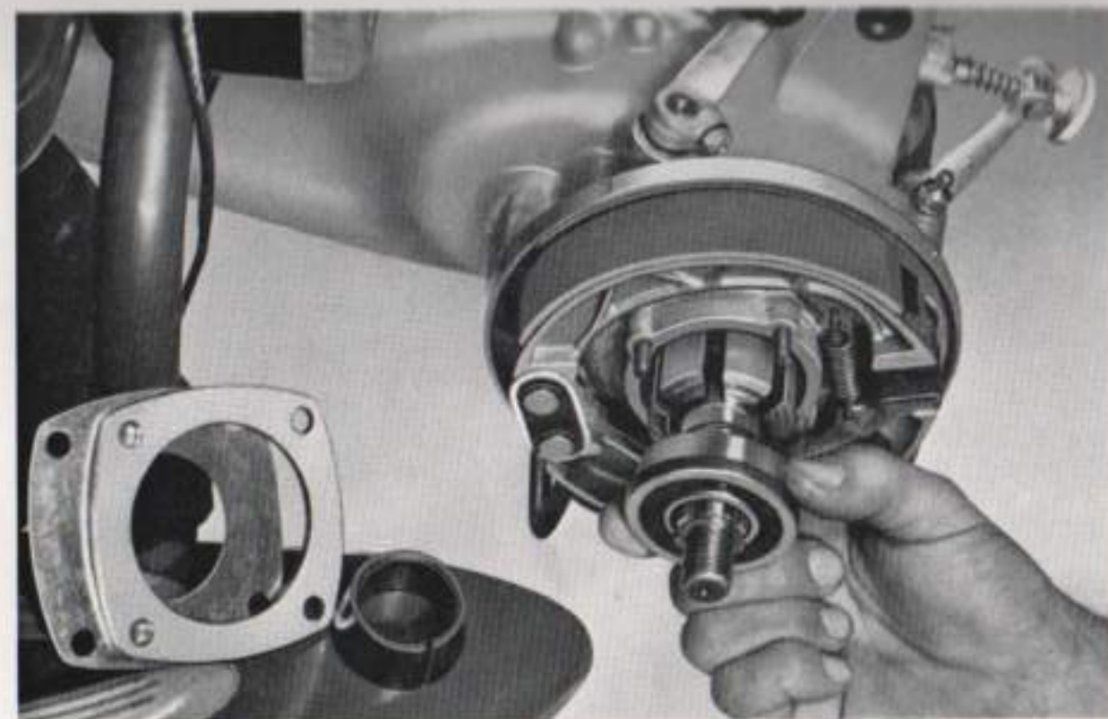
Axle driven towards the nearside to press out the bearing
