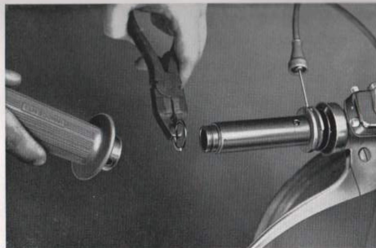
Dismantling the twist grip assembly
