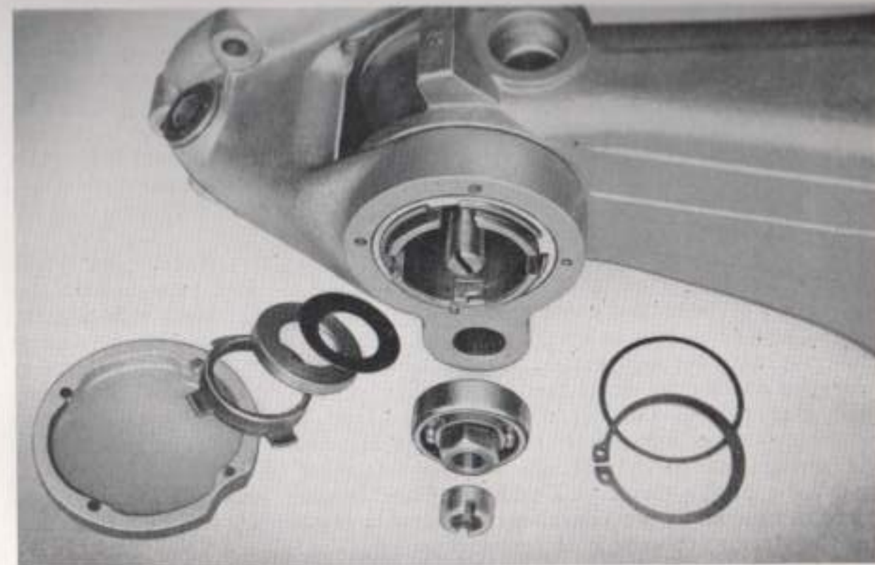
The pivot cover plate, bevel adjustment and bearing with retaining pieces removed
