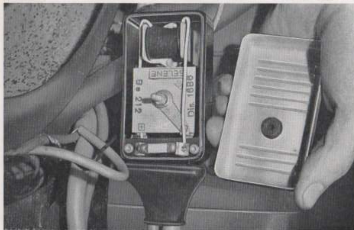
From top to bottom :— 5 amp. fuse, rectifier, impedance choke
