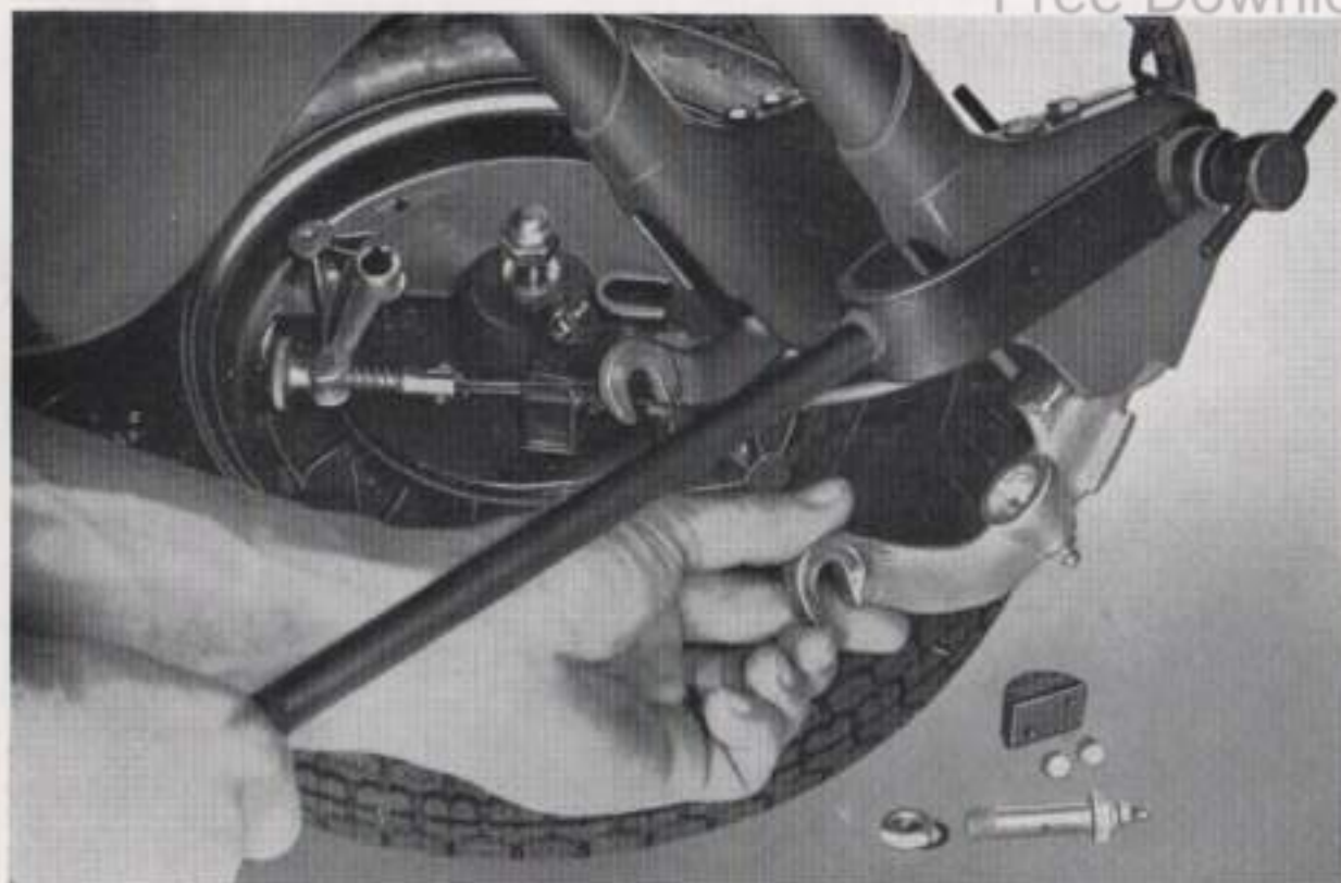
Compressing spring with tool 58021 to release trailing link
