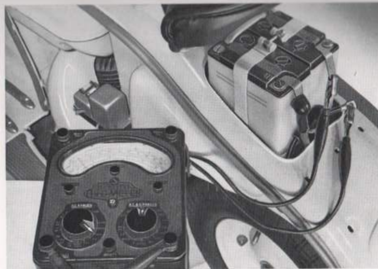
Measuring the leakage current from the batteries with the ignition switched off
