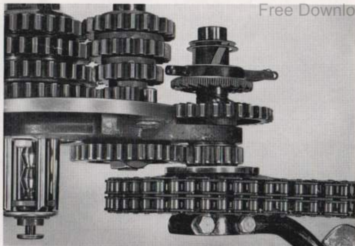
Face ratchet of kickstarter engages by action of helix as the shaft rotates
