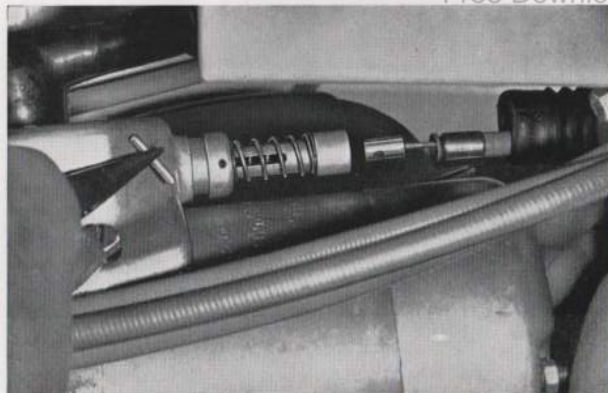
Re-fitting the cable of the starter switch of an LDA
