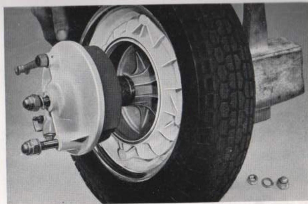
Wheel with extra bolt clamping back plate. Tapping out spindle
