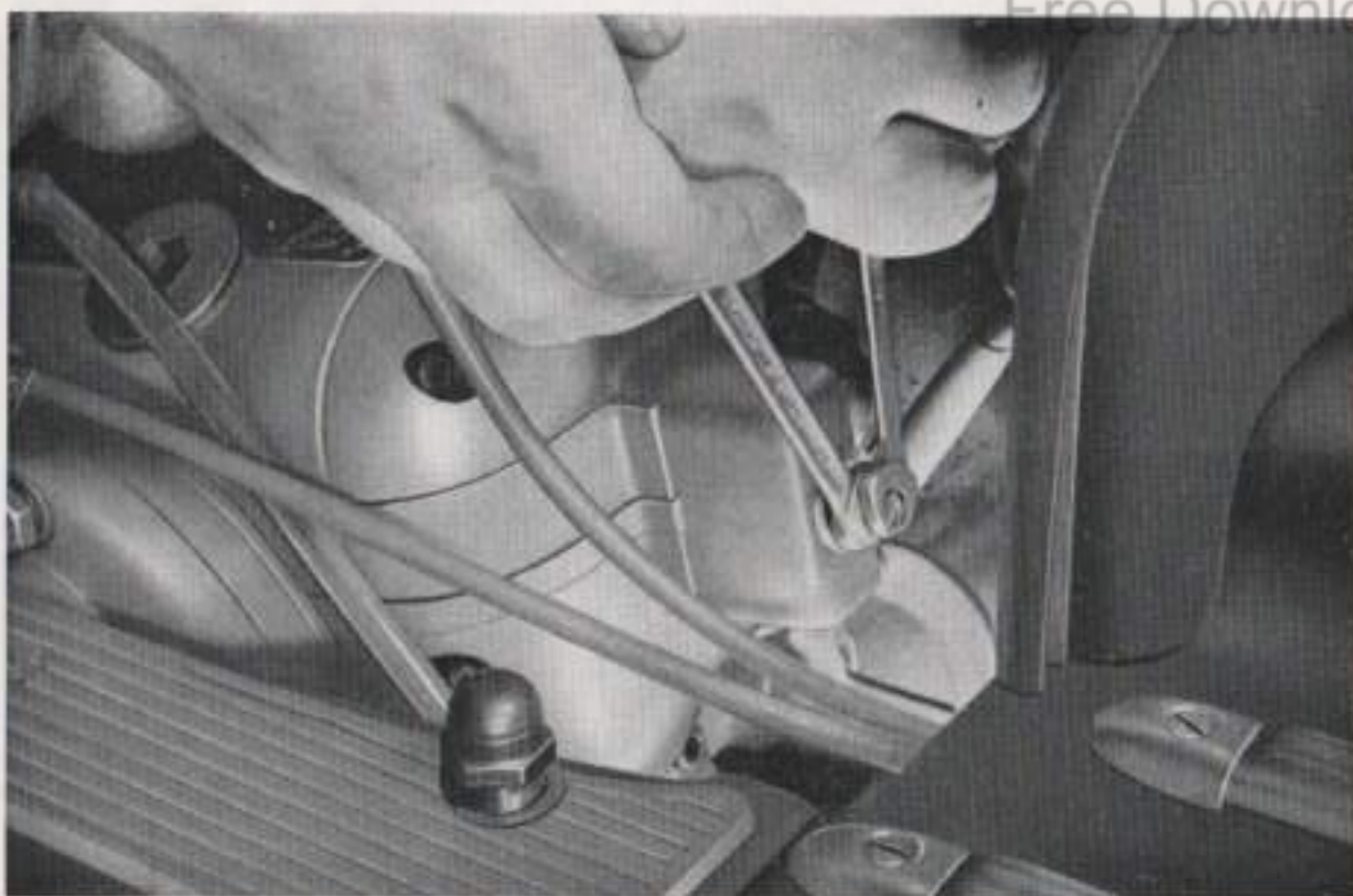
Adjusting the 8 mm. nuts on the clutch pull-rod
