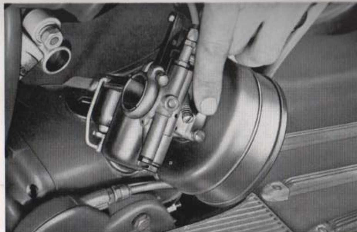
Idling mixture adjusting screw indicated, to the left the throttle stop screw
