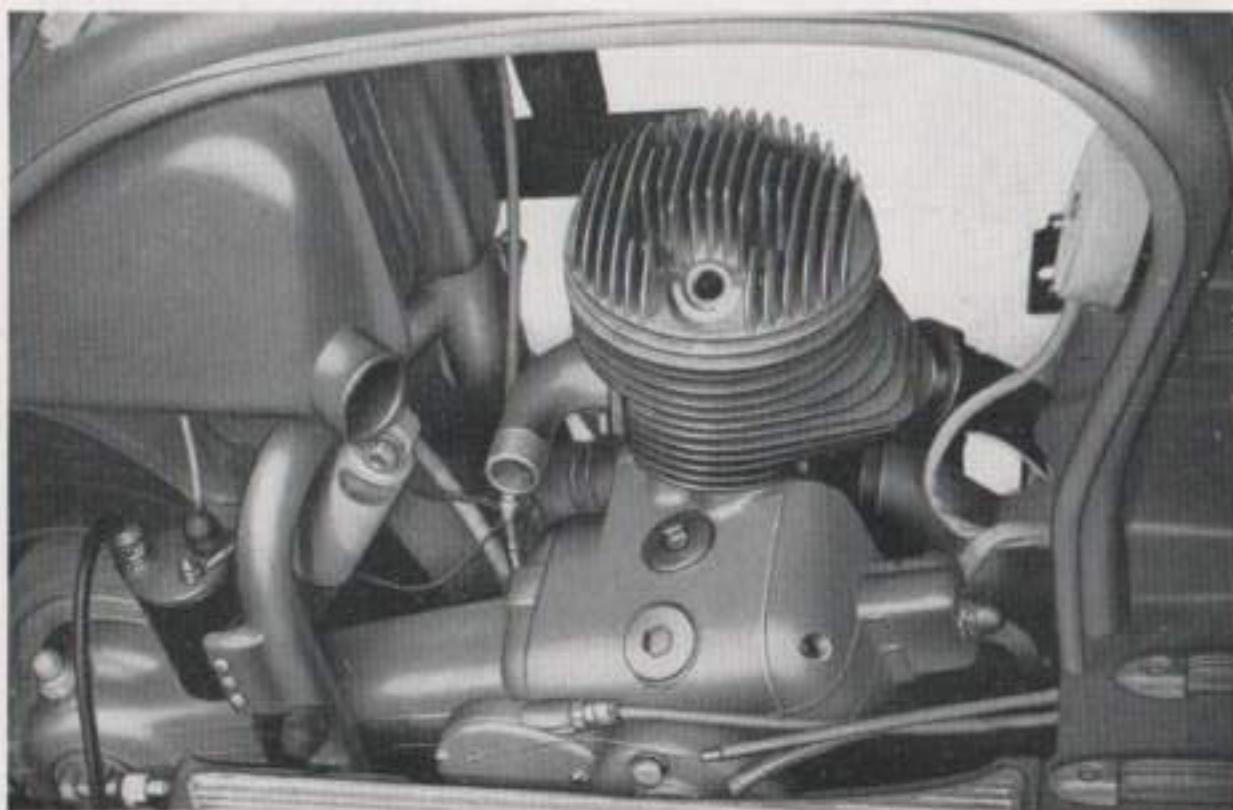
The cylinder exposed for dismantling and decarbonisation
